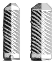
Production result of Counter-Deformed Spinal Cage showing the Displacement distribution; left: lateral view, right: frontal view mapped against original part design (Courtesy of Tangible Solutions).
