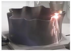
AM machine printing a part via DED process. (Ref BeAM machines, <u>www.beam-machines.com</u>).
