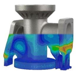
Deformations predicted as red zones in AdditiveLab via mechanical analysis. (Case study based on VTT pipe test geometry).
