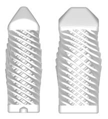
Simulation driven Counter-Deformed design of Spinal Cage via AdditiveLab; left: lateral view, right: frontal view.
